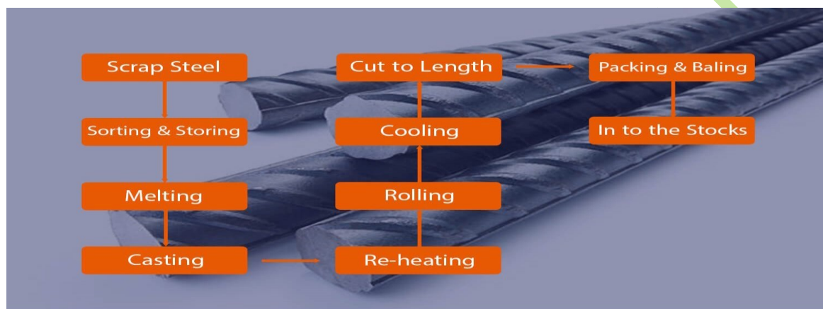
Production Process of Rolling Steel Rebar from Steel Scrap
